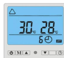
Picture: Timer set on. Heat pump to turn off in 6 hours.
